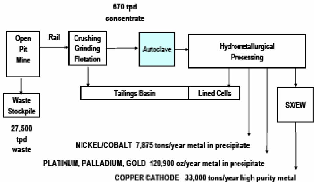
Metals emerge from the autoclave in a pregnant leach solution as copper sulfate, nickel sulfate and unstable, complex precious metals salts. Precious metals will be precipitated first into a rich sludge that can be sold to precious metals refineries.
